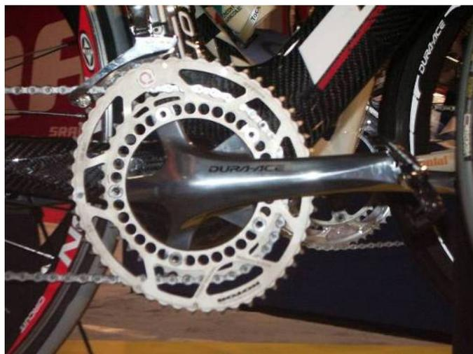
So, proceeding every OQC test, the Q regulation, or orientation of the crank in relation to the greatest diameter of the oval chainring, was determined for each individual cyclist.
